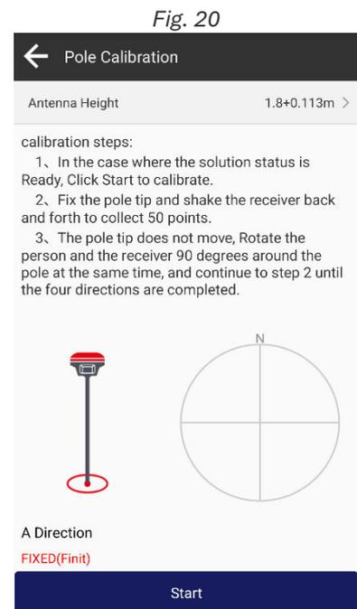
4. Fix the pole tip and shake the receiver back and forth to collect **50 points** (Fig.21)
